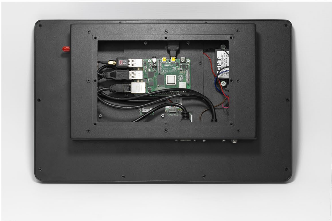
Interior of our case with Raspberry Pi 4 installed
