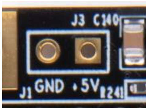
Power Interface on the Core Board
