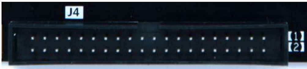
Figure 3-11-2: Expansion header J4 on the Carrier Board
