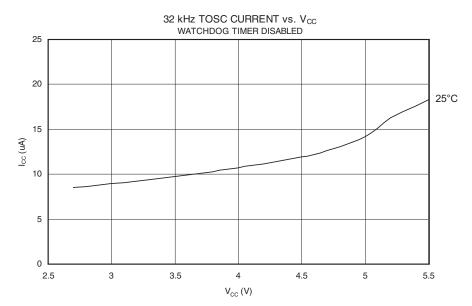
Figure 185. 32 kHz TOSC Current vs. V<sub>CC</sub> (Watchdog Timer Disabled)
