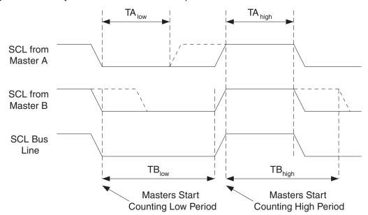
Figure 74. SCL Synchronization Between Multiple Masters
