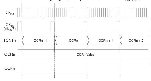
Figure 55 shows the setting of OCF2 and the clearing of TCNT2 in CTC mode.
