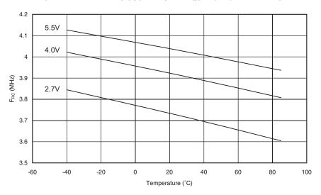
Figure 174. Calibrated 4 MHz RC Oscillator Frequency vs.  $V_{\rm CC}$
