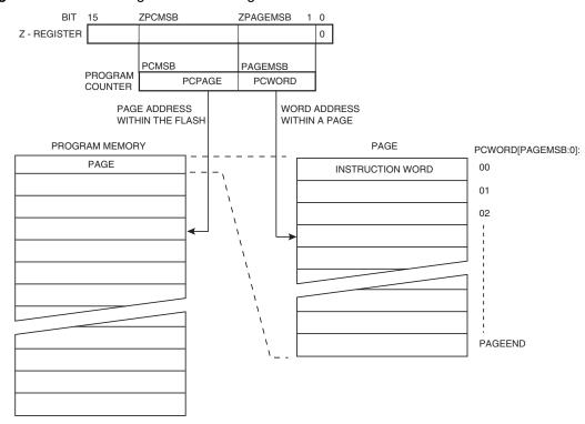
Figure 103. Addressing the Flash during SPM<sup>(1)</sup>
