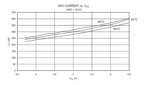
Figure 184. AREF External Reference Current vs.  $V_{\rm CC}$
