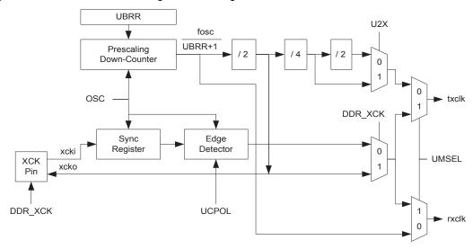
Figure 62. Clock Generation Logic, Block Diagram
