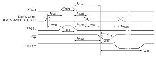
Figure 110. Parallel Programming Timing, Loading Sequence with Timing Requirements<sup>(1)</sup>
