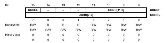
The UBRRH Register shares the same I/O location as the UCSRC Register. See the "Accessing UBRRH/UCSRC Registers" on page 152 section which describes how to access this register.
