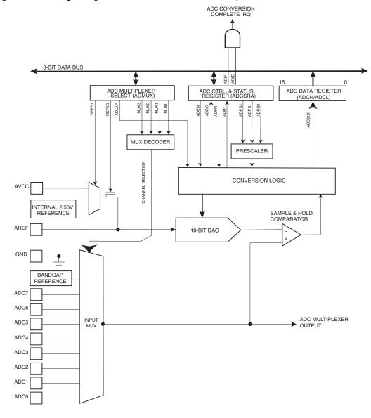
Figure 90. Analog to Digital Converter Block Schematic Operation
