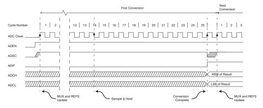
Figure 93. ADC Timing Diagram, Single Conversion
