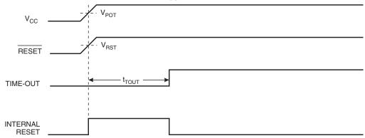
Figure 16. MCU Start-up, RESET Extended Externally
