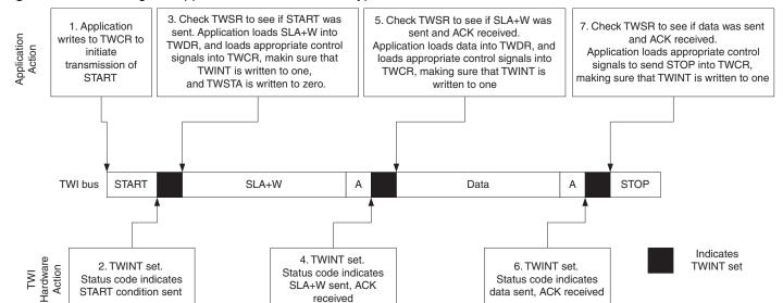
Figure 77. Interfacing the Application to the TWI in a Typical Transmission
