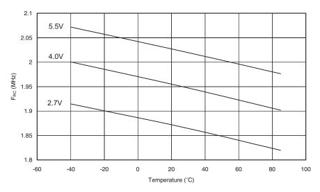
Figure 177. Calibrated 2 MHz RC Oscillator Frequency vs.  $\rm V_{\rm CC}$
