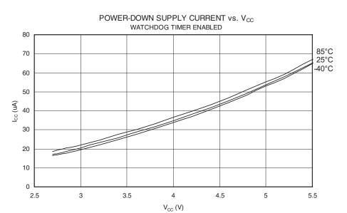
Figure 133. Power-down Supply Current vs.  $V_{\text{CC}}$  (Watchdog Timer Enabled)
