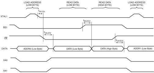
Note: 1. The timing requirements shown in Figure 109 (i.e., t<sub>DVXH</sub>, t<sub>XHXL</sub>, and t<sub>XLDX</sub>) also apply to reading operation.
