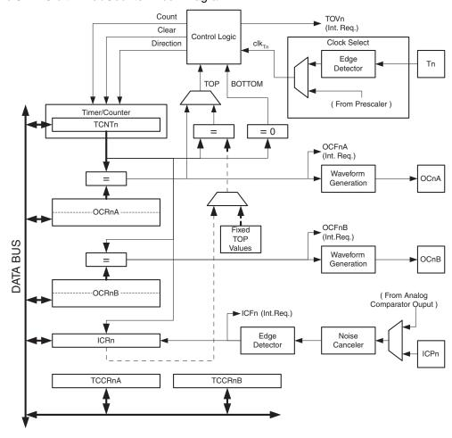
Figure 32. 16-bit Timer/Counter Block Diagram<sup>(1)</sup>
