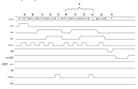
Figure 106. Programming the Flash Waveforms<sup>(1)</sup>
