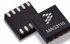
10-PIN DFN 2 mm by 2 mm by 0.85 mm CASE 2154-01
