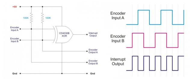
I was looking at how to write efficient code to convert these binary inputs into a simple "forward or backward" output. I ended up with a 2 dimensional array (matrix) that made the code quick and easy.
