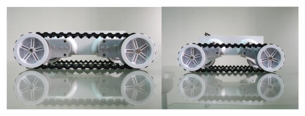
Each gearbox has an 87:1 ratio includes a hall effect quadrature encoder that gives 1000 pulses over 3 revolutions of the output shaft. The chassis can be upgraded to include four motors and encoders making it ideal for mecanum wheels.
