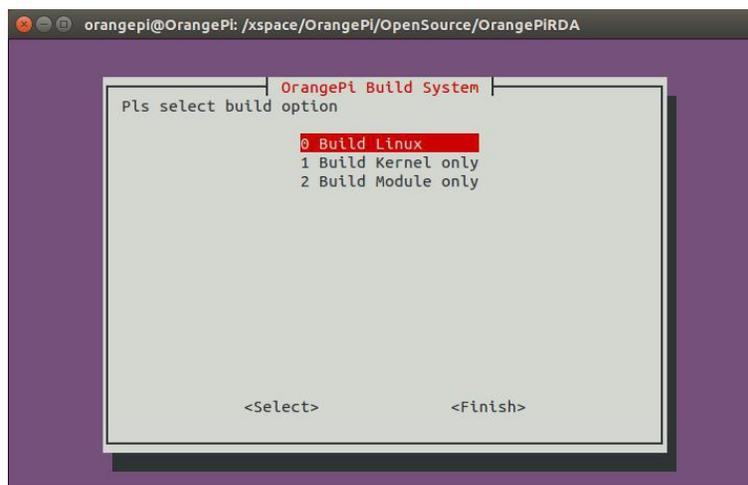
This version is only support the above three options. After selecting the corresponding option, the system would compile automatically.
