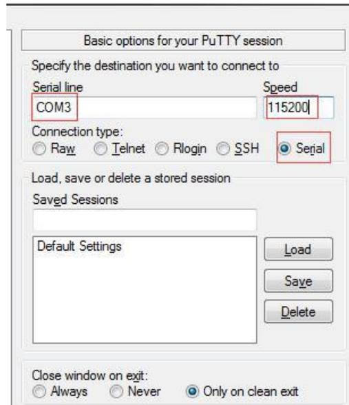
Serial port should set to the corresponding port number (COM5), the speed should set to 115200
