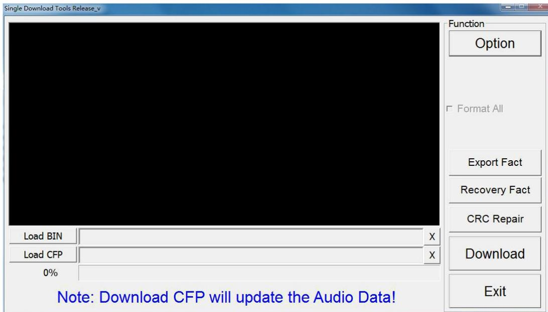
Click “load BIN” to import the image of NAND version into writing tool. After that, click Download button to download the image. Meanwhile, the tool is waiting for the download link of Orange Pi 2G-IOT.
