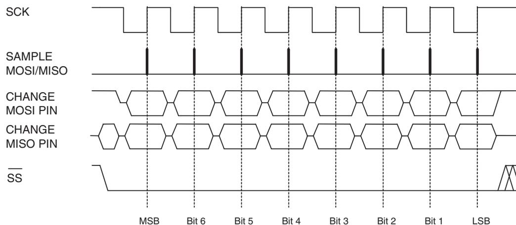
**Figure 6-2.** Data Byte Exchange – Timings
