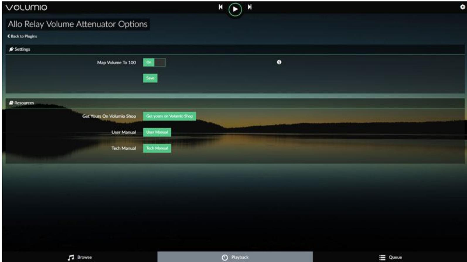
4. To use it with Piano, Piano 2.1, Boss DAC: simply plug it on top of them, and enable the DAC. It is suggested to set Volume of the DAC to 100 before enabling the Allo Relay Volume Attenuator Plugin and to set the Piano 2.1 in dual stereo mode.
