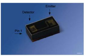
*Fig. 1: Photography and orientation of the SFH 7776.*
