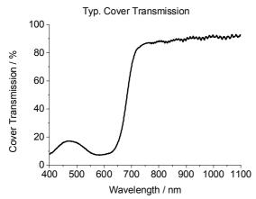
*Fig.* 18: *Typ. cover glass transmission characteristics.*
