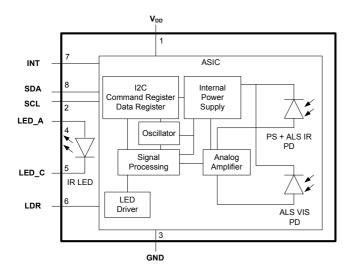
Fig. 2: SFH 7776 functional block diagram.
