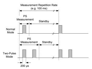
Fig. 7: LED drive current and timing during one proximity measurement cycle (two options are possible: normal and two-pulse mode).
