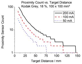
Fig. 9: Proximity sensor signal vs. target distance and LED drive current (reflector: Kodak Grey, 18 %, 100 x 100 mm<sup>2</sup>).
