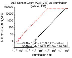
Fig. 6: Ambient light sensor count (ALS\_VIS) vs. illumination (different gain and integration time settings). The curves represent the maximum resp. the minimum sensitivity setting.
