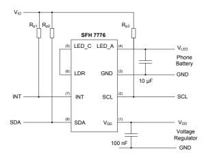
*Fig. 20: Recommended implementation into a mobile phone environment.*
