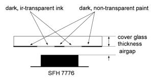
Fig. 13: Two-hole aperture design for minimum crosstalk level.
