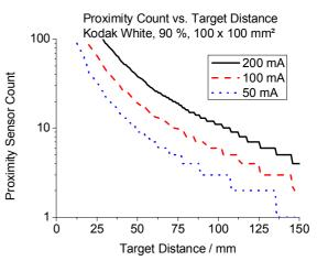
*Fig.* 8: *Proximity sensor signal vs. target distance and LED drive current (reflector: Kodak White, 90 %, 100 x 100 mm<sup>2</sup>).*
