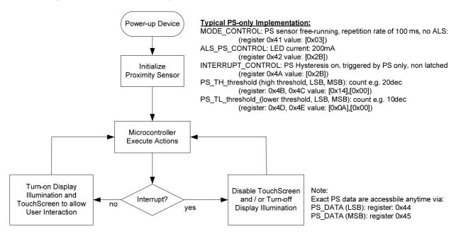
Fig. 22: Flowchart for a microcontroller based **proximity sensing** example.
