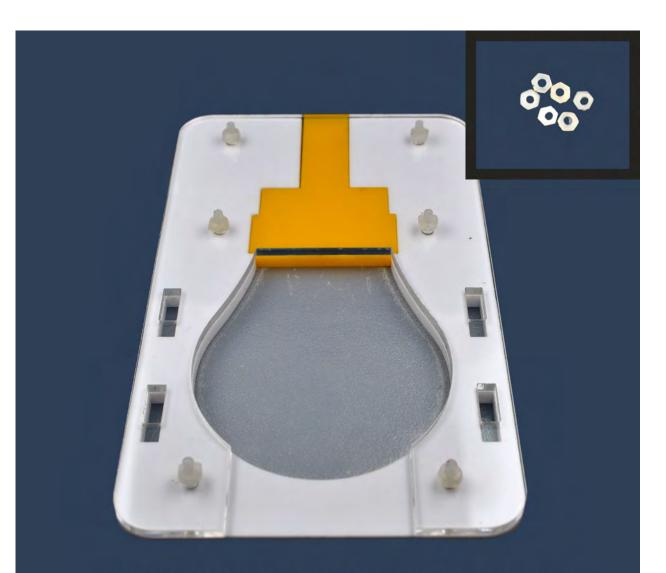
\* NOW LOCK ALL BOLTS WITH M3 NUTS AND TRIM THE EXCESS BOLTS OFF
