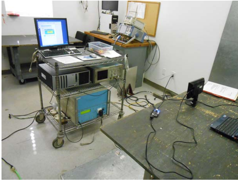
Test Setup – Voltage Dips and Interruptions
