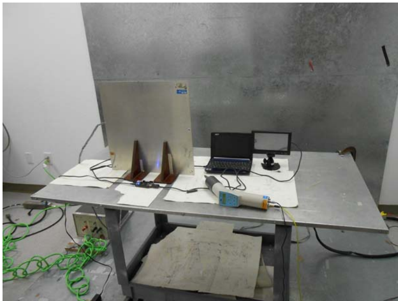
Test Setup – Electrostatic Discharge (ESD)
