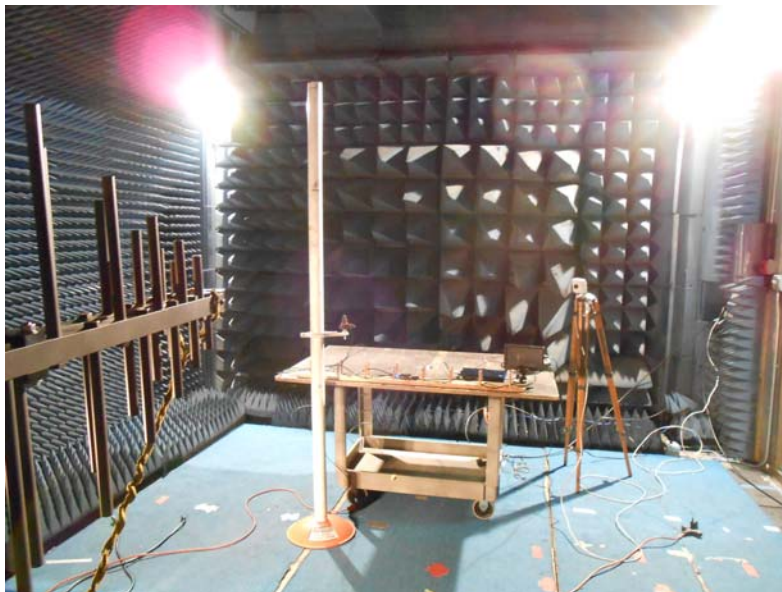
Test Setup – Radiated Disturbances
