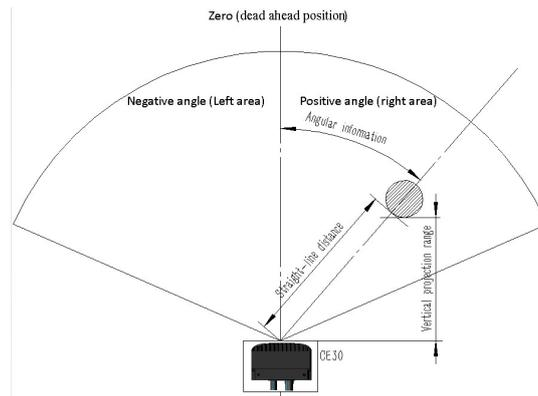
Figure 8 Testing Data Illustration (Top View)
