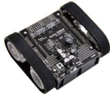
Fully assembled Zumo chassis with assembled Zumo Shield.
