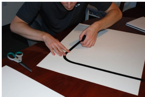
Stretch the tape very tightly, following the penciled curve.
