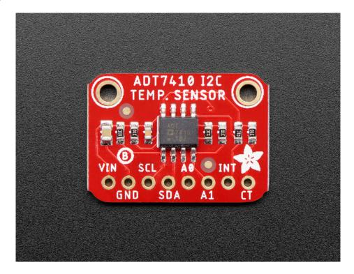
Analog Devices, known for their reliable and well-documented sensor chips - has a high precision and high resolution temperature sensor on the market, and we've got a breakout to make it easy to use! The **Analog Devices ADT7410** gets straight to the point - it's an I2C temperature sensor, with 16-bit 0.0078°C temperature resolution and 0.5°C temperature tolerance. Wire it up to your microcontroller or single-board computer to get reliable temperature readings with ease
