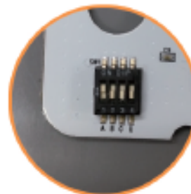
'A' ON A: BLE Serial Data Mode while OFF, BLE Advertise Mode while ON
