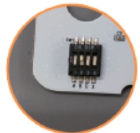
'B' ON B: 32-channel Measurement Standard Mode while OFF, Cushion Sensor Compensation Mode while ON
