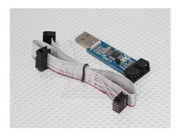
Connect your Programmer's 6 pin socket to the ISP header on the board. Pin 1 on the ISP header is usually marked with a small triangle. Then connect the a 5V DC power source to the PCB pins.
