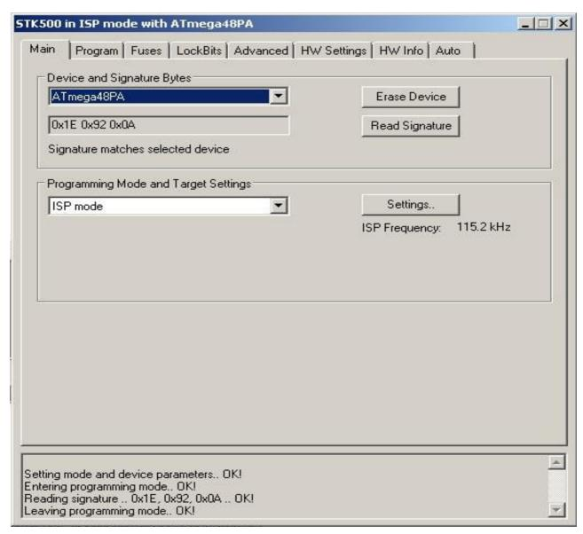
Also make sure that the target board or PCB is powered (You can check this by clicking on the HW Settings tab and checking if the programmer can see any voltage).
