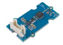
This accelerometer has a wide measurement range of -100g to +100g and is an ultralow, high frequency, high G, industrial grade MEMS accelerometer, based on ADXL10001.
