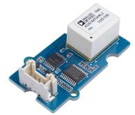
This has a 6-Axis Miniature MEMs sensor, which includes a triaxial gyroscope and a triaxial accelerometer. Also, each inertial sensor in the ADIS16470 combines with signal conditioning that optimizes dynamic performance.
