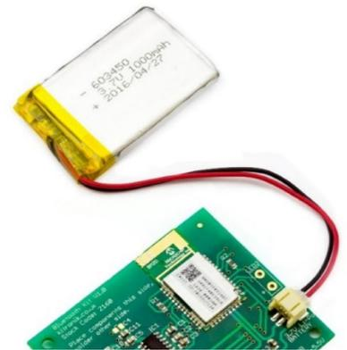
**It is important that the polarity of the battery is correct.** It is important that the polarity of the battery is correct. The JST connector on the PCB labelled CON2 is used to connect the battery. The pin next to the bottom right mounting hole is the positive battery connection (as shown in the picture right). This should be checked before connecting a battery.
