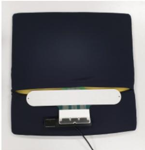
Connect the Micro USB cable to the shield.
