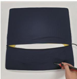
If the cable folds inside the cushion, it may cause a measurement error. Make a small hole on the cover.
