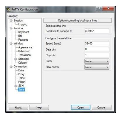
3. Open category Session and switch connection type to Serial. Value in the field Serial line and Speed should update. There is an option to save configuration. You can name configuration in field under Saved sessions then press the Save button. The list will update. To use one of saved configurations simply check one from the list then press Load button.
