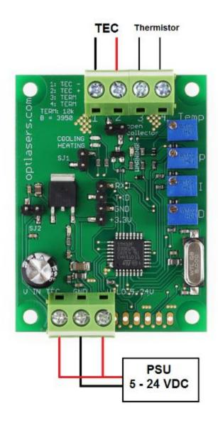
3. Using one PSU with **closed SJ2**:
