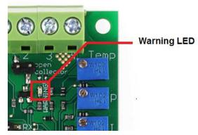
5. If the measured temperature lies between +45°C and Tmax, the WARNING LED is flashing. The open collector output (OC) is not connected to ground. The PID regulator works normally (unless the overriding limit mentioned before is exceeded).
