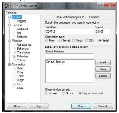
4. After setting up the session parameters click the **Open** button. The terminal window will show up. If you want to make sure TEC 8A-24V-PID is connected properly you can reset the device. Simply disconnect it from the power supply and after couple seconds connect again. You will receive initialization info from the device (shown below).
