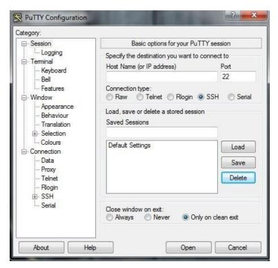
Open category Connection->Serial. Make sure transmission parameters are set properly (look for chapter TEC 8A-24V-PID Connectivity and check parameter values). In field Serial line to connect to write the name (COM) of the USB to UART converter shown in the device manager operating system (Figure 2.)
