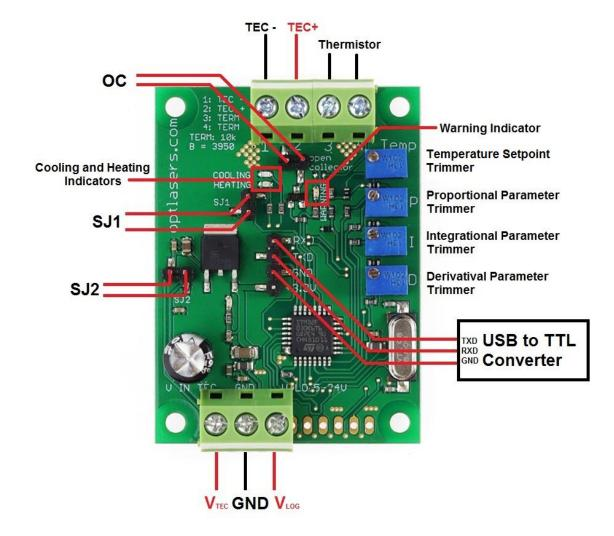
Figure 1. TEC 8A-24V-PID Connection scheme
