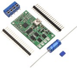
Simple High-Power Motor Controller 18v15 or 24v12, partial kit with included hardware.
