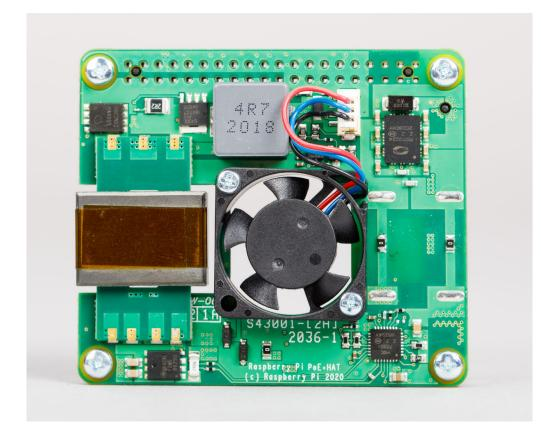
The Raspberry Pi PoE+ HAT is an add-on board for Raspberry Pi computers with PoE pins, including Raspberry Pi 3B+ and Raspberry Pi 4. It is used to power Raspberry Pi via an Ethernet cable, provided that power-sourcing equipment is installed on the Ethernet network. The HAT also includes a fan that will cool the Raspberry Pi processor.
