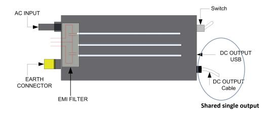
Chassis Ground always connected to Earth connector
