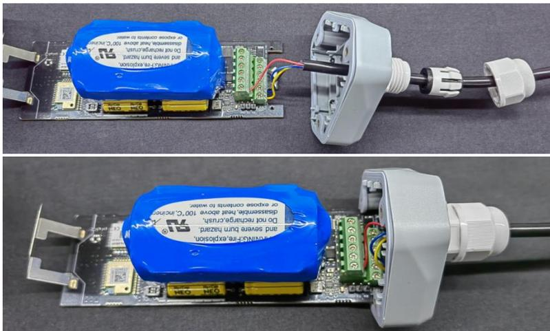
3. Tighten the screws and screw caps to check the waterproofing. If the wire diameter is too thin, add waterproof tape for winding.
