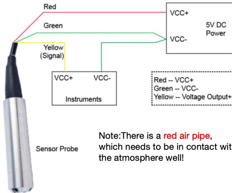
1. Pass the sensor cable through the bottom cover and connect it to the base of the Data Logger according to the wire sequence requirements;
