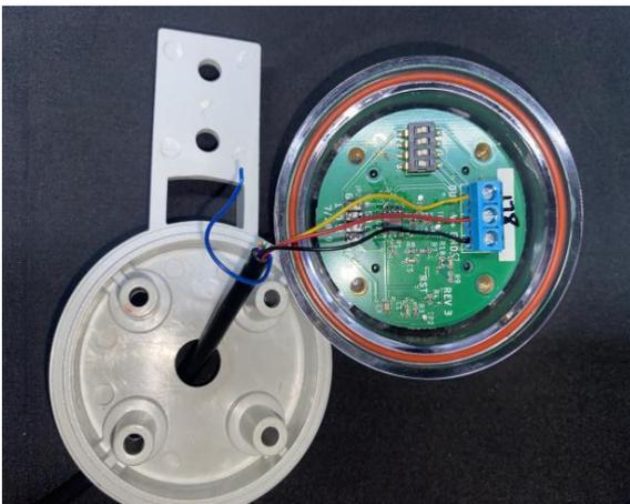
2. Turn the DIP Switches 1 of the rain sensor S1 base to the ON, turn the switch 2 to the OFF , and turn the 3 and 4 to the OFF;
