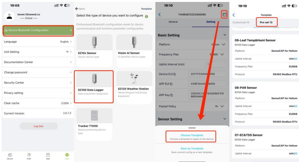
Using pre-set template set sensor via SenseCAP Mate App
