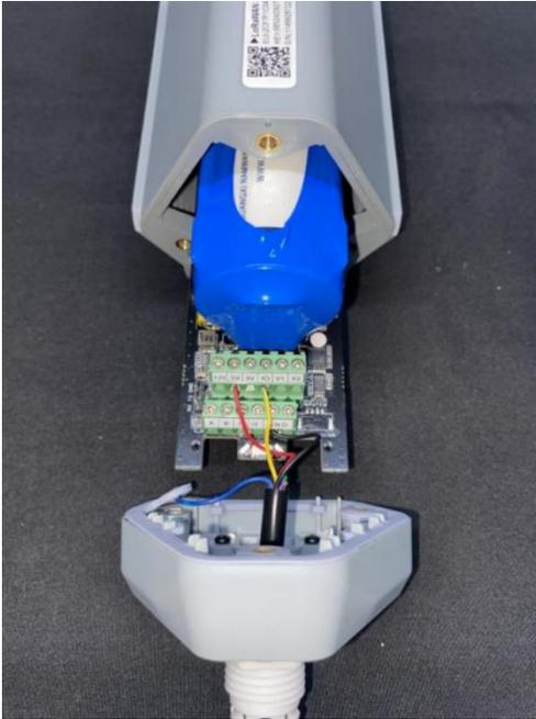
5. Connect the upper cover, rubber ring and screw cap in sequence
