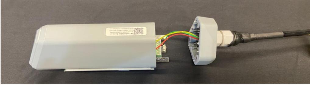
3. Tighten the screws and screw caps to check the waterproofing. If the wire diameter is too thin, add waterproof tape for winding.
