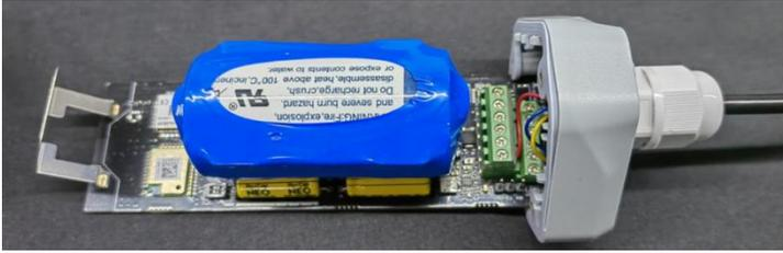
3. Tighten the screws and screw caps to check the waterproofing. If the wire diameter is too thin, add waterproof tape for winding.
