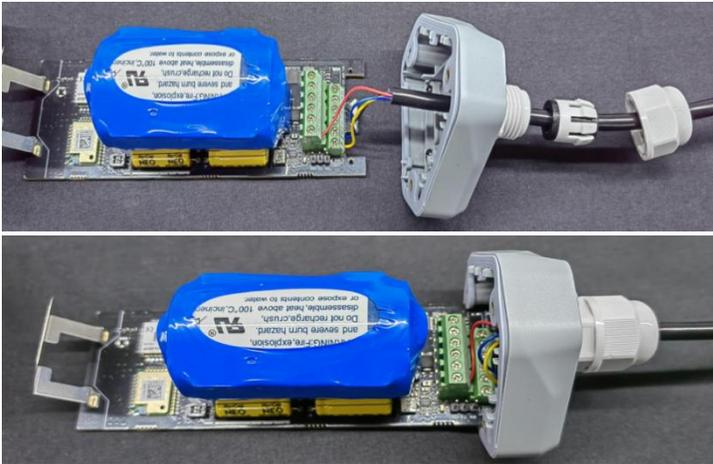
3. Tighten the screws and screw caps to check the waterproofing. If the wire diameter is too thin, add waterproof tape for winding.
