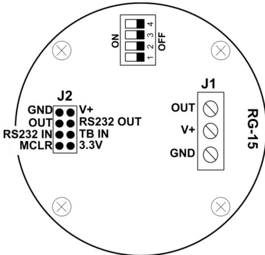
1. Unscrew four screws, take down the cover. Pass the 8 pin wire through the bottom cover and connect it to the base of the J1 according to the wire sequence requirements;
