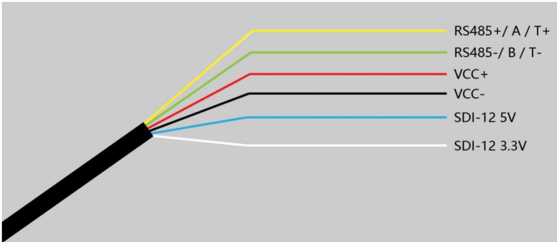
1. Pass the S4 sensor cable through the bottom cover and connect it to the base of the Data Logger according to the wire sequence requirements;
