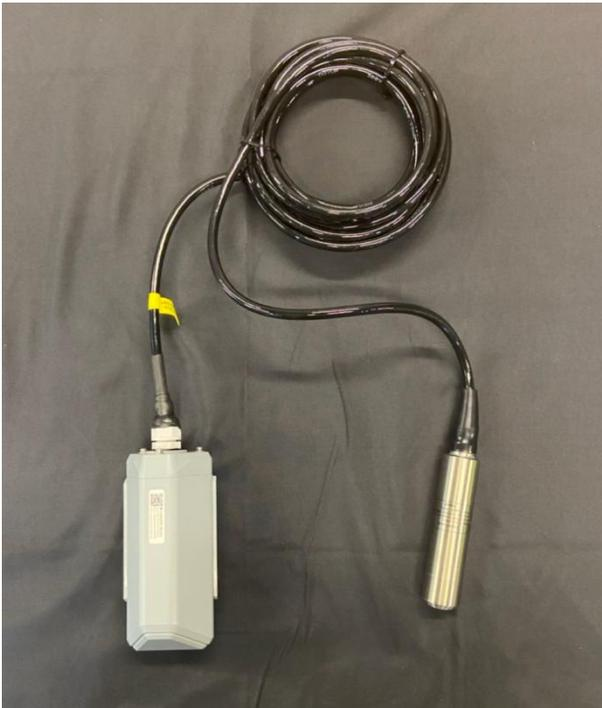
**\*Note:** When assembling the device, it is necessary to install the waterproof pad of the Data Logger and the adapter box, and tighten the screw cap and screw, otherwise the waterproof effect of the device may be affected!
