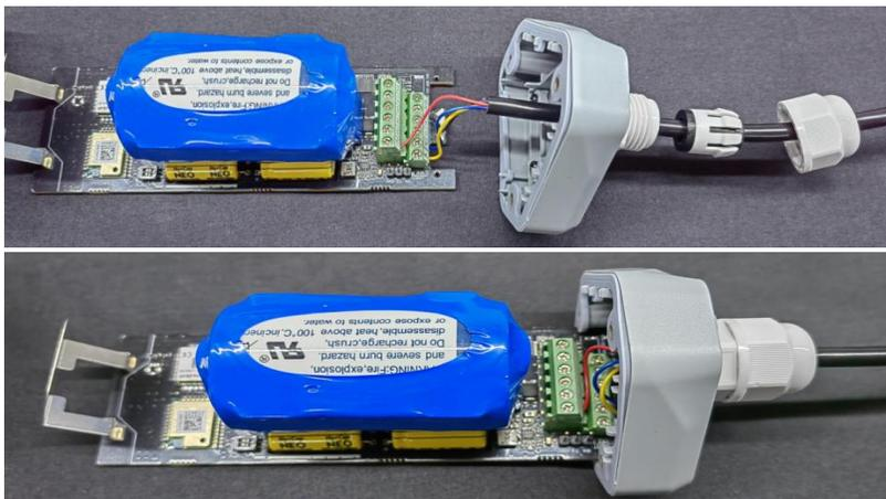
3. Tighten the screws and screw caps to check the waterproofing. If the wire diameter is too thin, add waterproof tape for winding.
