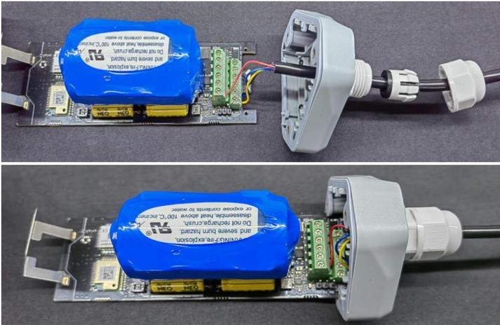
6. Tighten the screws and screw caps to check the waterproofing. If the wire diameter is too thin, add waterproof tape for winding.
