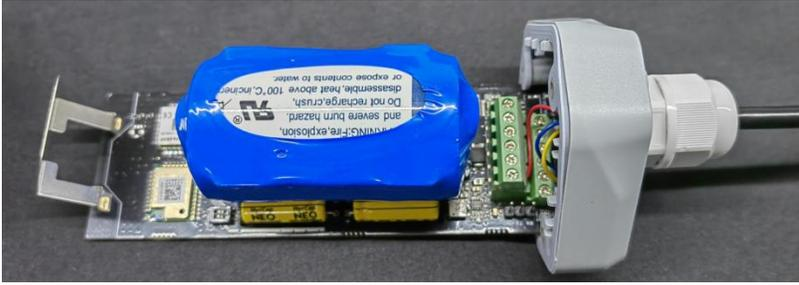
3. Tighten the screws and screw caps to check the waterproofing. If the wire diameter is too thin, add waterproof tape for winding.
