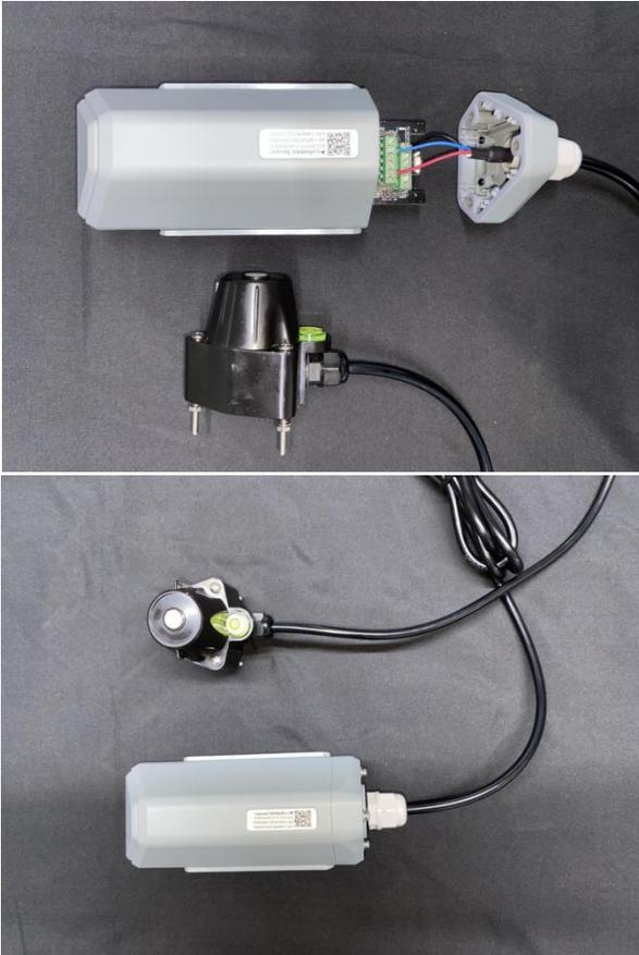
**\*Note:** When assembling the device, it is necessary to install the waterproof pad of the Data Logger and the adapter box, and tighten the screw cap and screw, otherwise the waterproof effect of the device may be affected!
