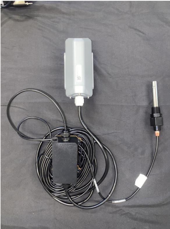
**\*Note:** When assembling the device, it is necessary to install the waterproof pad of the Data Logger and the adapter box, and tighten the screw cap and screw, otherwise the waterproof effect of the device may be affected!
