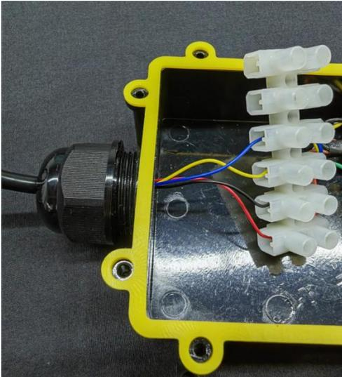
4) Connect the M12 sensor wire to the junction box.
