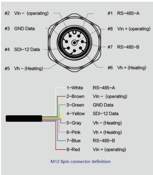
The device adopts an M12 8-pin connector, the different colored pins provide power and data communication (as shown in the above diagram).
