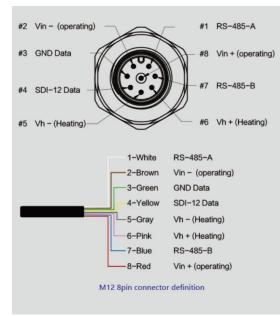
The device adopts an M12 8-pin connector, the different colored pins provide power and data communication (as shown in the above diagram).
