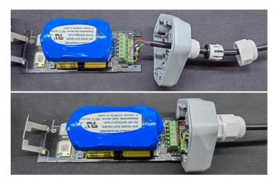
**3. Tighten the screws and screw caps to check the waterproofing**. If the wire diameter is too thin, add waterproof tape for winding.
