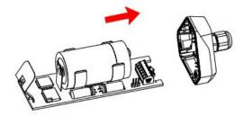
3. Remove the thread cap and pass it through the cable of the sensor, pass it through the bottom cover, and connect it to the wiring terminal.
