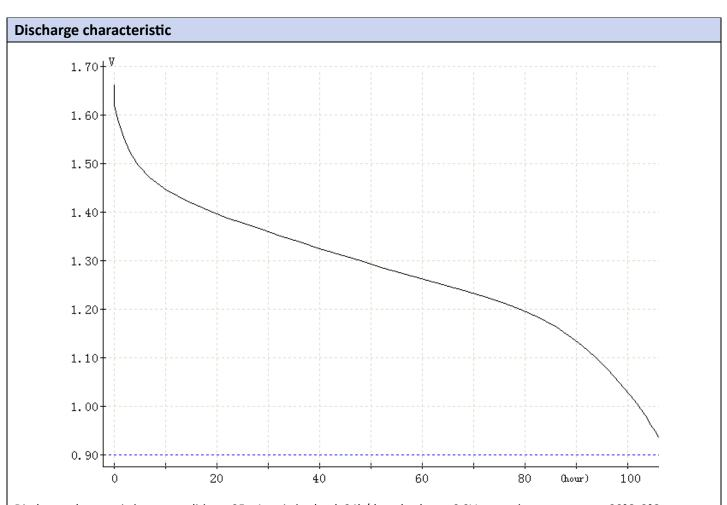
$Discharge\ characteristic\ test\ conditions:\ 25 mA\ resistive\ load,\ 24 h/d,\ end\ voltage:\ 0.9 V,\ operating\ temperature\ 20^{\circ}C\pm 2^{\circ}C$
